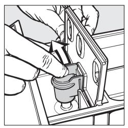
Remove the siphon tube from compartment <sup>(B)</sup>.
